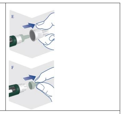
Step 2 Check the flow before each injection
